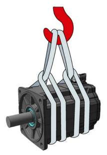
Figure 7-1 Lifting and transporting with lifting slings (example diagram)
